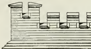
PARAPET: MODERN PATTERNS IN BRICKWORK, WHICH MUST BE CAREFULLY LAID IN STRONG CEMENT MORTAR.
